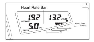
Note: The console can display speed and distance in either miles or kilometers. The letters "MPH" or "Km/H" will appear in the right display to show which unit of measurement is selected. To change the unit of measurement, see THE IN-FORMATION MODE/DEMO MODE on page 19. For simplicity, all instructions in this section refer to miles.
